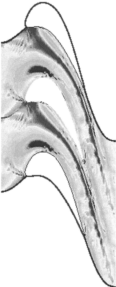
Fig. 2a Lumped deterministic energy at midspan obtained from third-order TURBO code. 4
