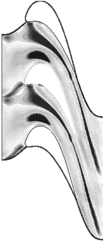
Fig. 2b Lumped deterministic energy at midspan obtained from the linear unsteady TACOMA code. 4
